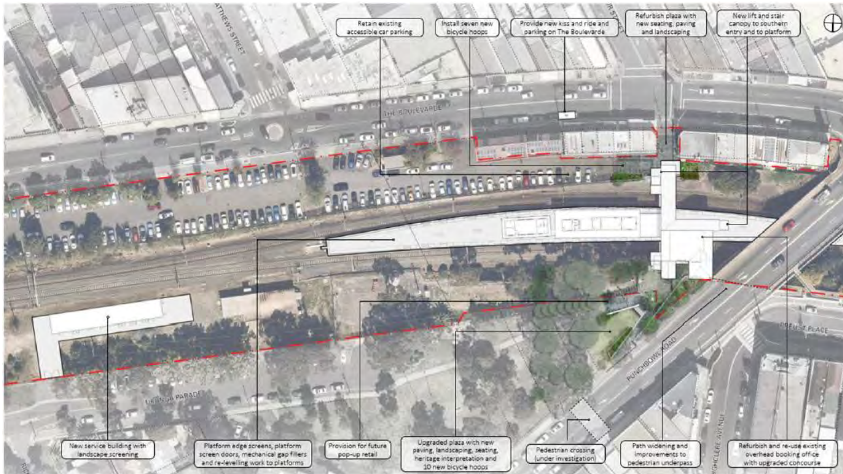
Figure 3 Sydney Metro Punchbowl Station upgrades
