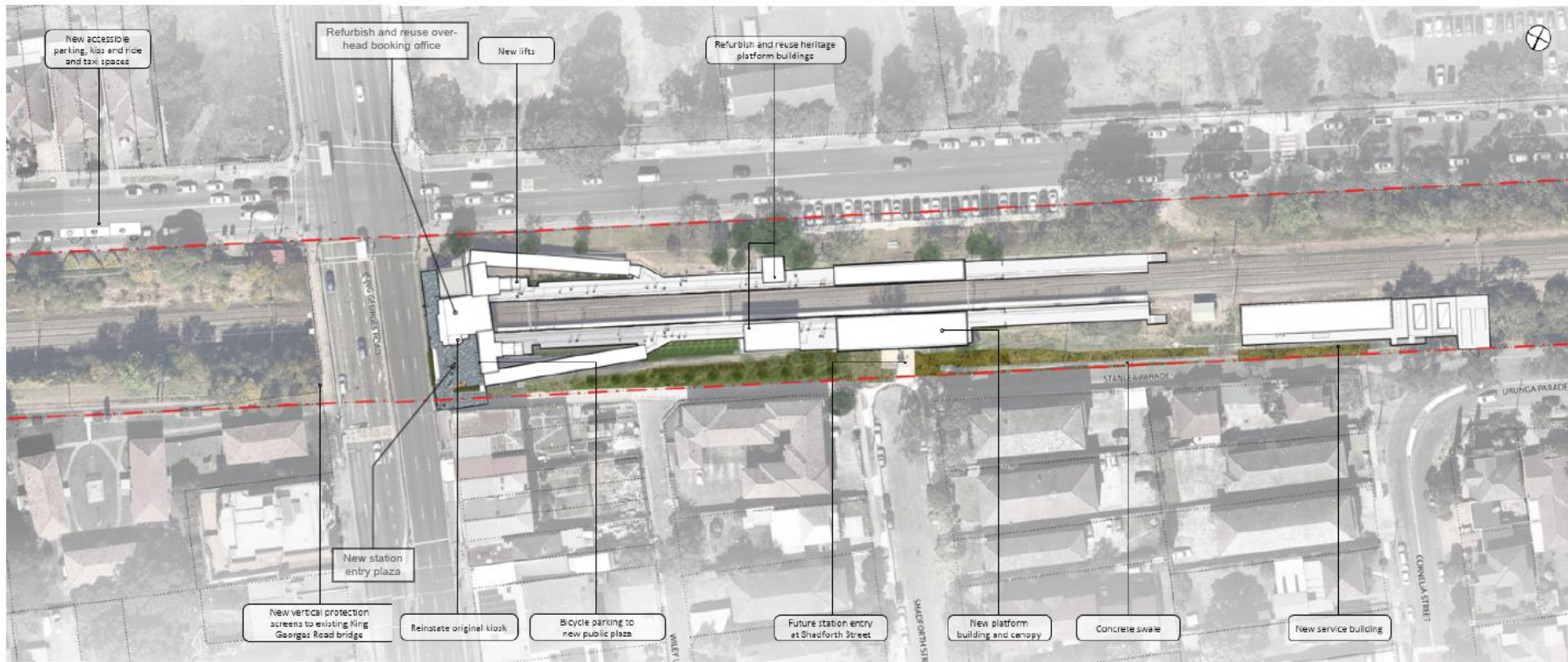
Figure 4 Sydney Metro Wiley Park Station upgrades
