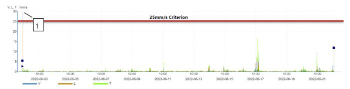
**Figure 8 –** Unattended vibration monitoring location for 2 Hopetoun Street (shed) between 02/06/2022 and 22/06/2022
