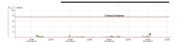
Figure 9 - Unattended vibration monitoring at Punchbowl Station between 24/09/2022 and 27/09/2022
