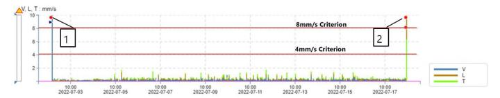
Figure 3 - Unattended vibration monitoring results for 3A Commons Street between 02/07/2022 and 18/07/2022
