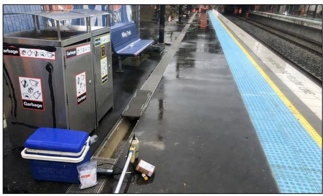
Photograph 7. Aco drain check – tap water test. Date: 5 October 2022.
