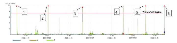
Figure 2 – Unattended vibration monitoring results for 5 Railway Street between 20/04/2022 and 04/05/2022
