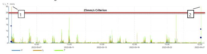
Figure 5 – Unattended vibration monitoring location for 2 Hopton Street between 04/05/2022 and 27/05/2022
