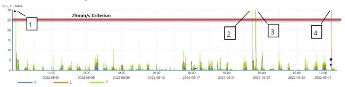
Figure 4 – Unattended vibration monitoring results for 3 Railway Street between 27/04/2022 and 02/06/2022
