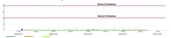
**Figure 10 –** Unattended vibration monitoring at 3A Commons Street, Hurlstone Park between 24/09/2022 and 27/09/2022.
