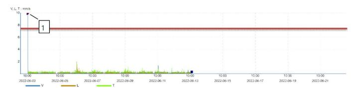
**Figure 8 –** Unattended vibration monitoring location for 2 Hopetoun Street (building) between 03/06/2022 and 22/06/2022
