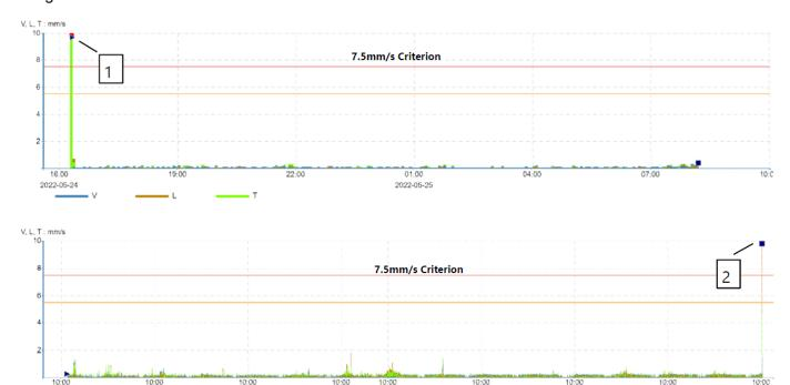
Figure 6 - Unattended vibration monitoring location for 3A Commons Street between 04/05/2022 and 27/05/2022
