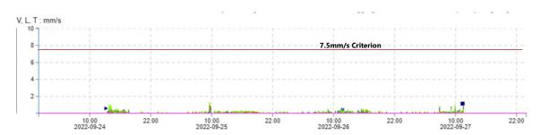
It can be seen in Figure 4-1, that the vibration levels produced from the vibration intensive works in the proximity of the station lift at Punchbowl Station are below 7.5mm/s.
